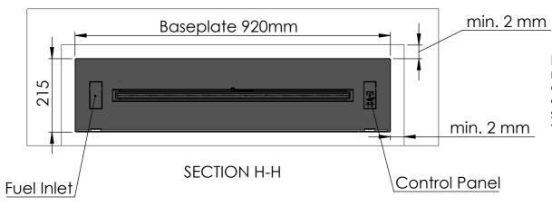
Please Note, if using the minimum required dimensions for the wall cutout, the wall in front of the safety chamber becomes very thin, only 7,5mm.
